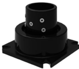
The 3" Base kit includes one SlowStop® rebounding base and anchors. You must supply your own pipe. Pipe required: ANSI schedule 40 nominal 2.5" pipe with outside diameter of 2.88".
