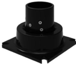
The 4" Base kit includes one SlowStop® rebounding base and anchors. You must supply your own pipe. Pipe required: ANSI schedule 40 nominal 3.5" pipe with outside diameter of 4".
