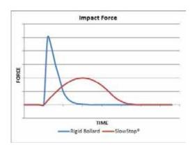
SlowStop® is designed as a frangible, easily maintained, modular system that prevents damage to concrete and structural floors. The system is made up of four main components: The post (standard schedule 40 pipe), base, adapter, and the energy absorbing elastomer. Each piece is modular and easily replaced should damage occur. The system is installed using four to eight concrete anchor screws to secure the unit to concrete.
