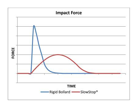
This leads directly to the most important advantages of the SlowStop® Bollard
