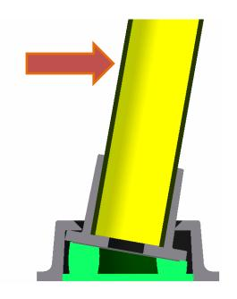
SlowStop Bollards® are designed in a variety of sizes, each of which is appropriate for various expected collision speeds and masses. Further, they are
