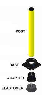
temperature. The steel pipe which serves as the bollard post is a typical steel pipe inserted into the adapter. In the US, standard ANSI schedule 40 pipe is use to give the end user the flexibility to weld fencing using standard components if necessary. Concrete fill is not required inside the bollard pipe, though is permitted. In fact, sign posts can be inserted into the post and concrete filled in place.
